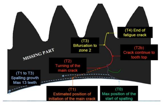
Figure 5: An estimate of the fracture sequence.
